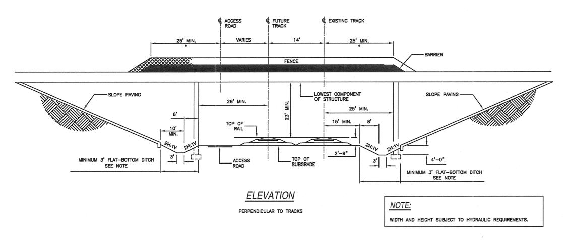
\* THE LIMITS OF THE FENCE WITH BARRIER RAIL SHALL EXTEND TO THE LIMITS OF RAILROAD RIGHT-OF-WAY OR A MIN. OF 25 ft BEYOND THE CENTERLINE OF THE OUTERMOST EXISTING TRACK, FUTURE TRACK OR ACCESS ROADWAY. WHICHEVER IS GREATER.
