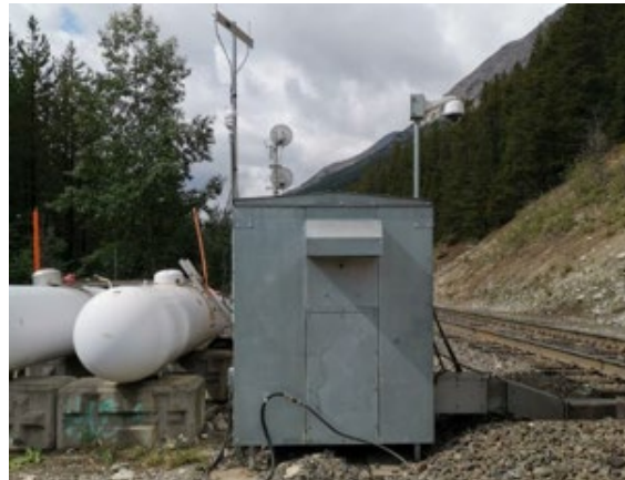
CPKC has installed weather stations between Calgary, Alta. and Swift Current, Sask. to obtain more pinpointed wind gust data. This data helps drive informed operational decisions, reducing the risk of train derailments during winter polar vortex conditions.
